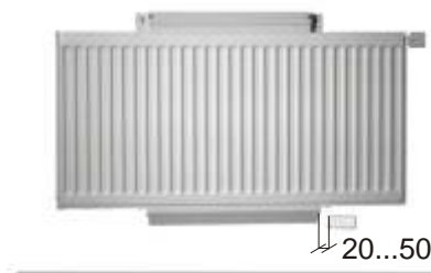
Correct location for the temperature sensor of the thermostatic valve is below the radiator at a distance of 20...50 mm from the supply air device
