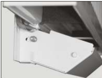
PURMO Air service cover is opened for cleaning and replacing the air filter. Duct surfaces should be dry cleaned using a vacuum cleaner or brush.
